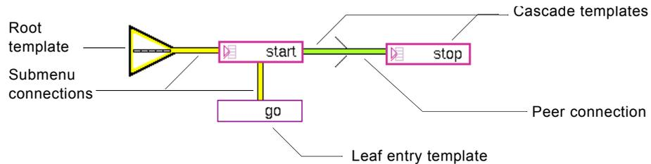
The only difference between the specification of a menu bar and the specification of a popup menu is the type of root template used. For a menu bar use a **Menu Bar template** and for a Popup menu use a **Popup Menu template**.
