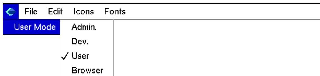
GMS automatically positions a menu bar at the top of the G2 window. If the window is not wide enough to show all menu entries in one row, GMS automatically wraps the menu onto additional rows as needed.
