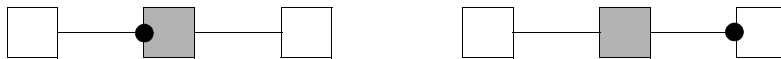
The most basic type of block simply passes work objects to the downstream block.
