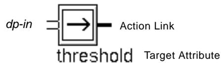
The Set Attribute block sets the value of an attribute to the block's input data value. Specify the object whose attribute you would like to set by connecting the Set Attribute block's action link to it. You can connect the action link to any G2 object or block. Specify the attribute you would like to set by setting Target Attribute to its name.
